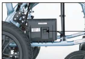
Main power switch (Manual mode switch)
