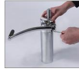
2.Install the foot lever on the hydraulic pump and tighten the short hex socket screw with a wrench.
