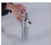
1. Take out the product and all accessories, install the hydraulic pump cover, screw the small screws on the cover.
