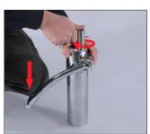
4.If the hole at the upper end of the solid shaft of the liquid pump rod is not in the middle position, press the foot rod to the very bottom and do not release it. At the same time, rotate the solid shaft to align the hole with the small screw on the decorative cover. At the same time, press the solid shaft to the very bottom and then release the foot rod.
