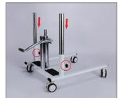
7.Insert the two thick round tubes into the mounting holes of the base frame, and screw in the black twist screws to press the round tubes tightly.
