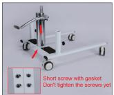
6.Install the hydraulic pump on the bottom rack, insert 4 M8\*30 screws into the gasket, and screw in from the bottom. (Don't tighten the screws yet)
