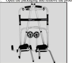
2. Hold the PVC handles on both sides with both hands, then pull them outward. When you hear a "snap" sound, the walking aid will fully ope:
