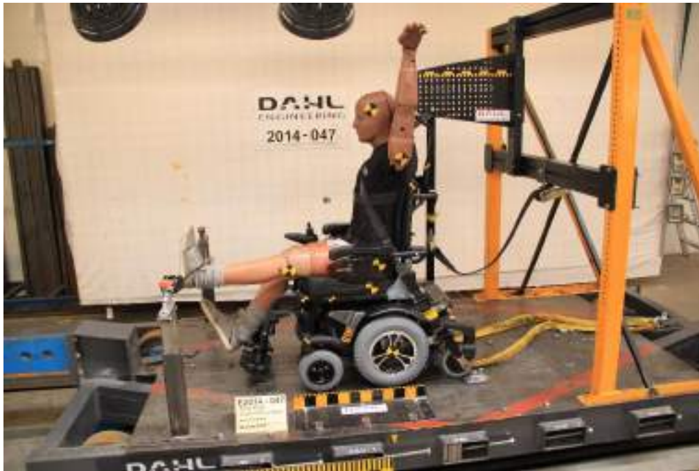
Morgan crash test using Dahl Docking station.
