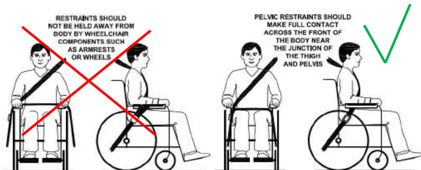
picture of improper belt fit
